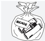
If the instrument is wet, it must be dried prior to storage.
