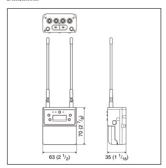
$63 \times 70 \times 35 \text{ mm } (2^{1}/_{2} \times 2^{7}/_{8} \times 1^{7}/_{16} \text{ in.})$ (width/height/depth)
