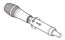
**3** Insert two new AA batteries into the battery compartment with ⊕ and ⊖ polarities in the correct orientation.
