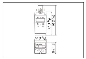
$38 \times 98 \times 38 \text{ mm} (1^{1}/_{2} \times 3^{7}/_{8} \times 1^{1}/_{2} \text{ in.})$  (width / height / depth) (including the audio input connector) Approx. 139 g (4.9 oz)
