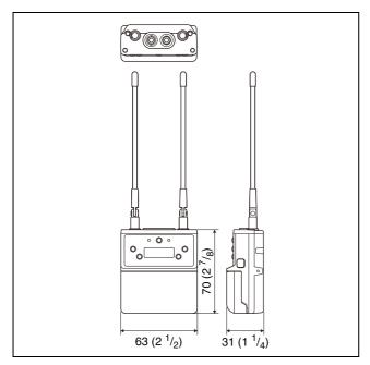
$63 \times 70 \times 31 \text{ mm} (2^{1}/_{2} \times 2^{7}/_{8} \times 1^{1}/_{4} \text{ in.})$ (width / height / depth) (excluding antenna) Approx. 131 g (4.6 oz) (excluding batteries)
