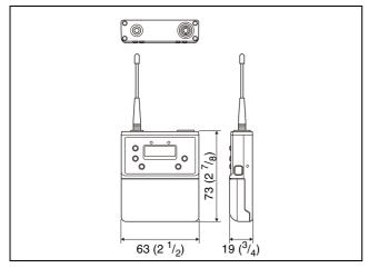
$63 \times 73 \times 19 \text{ mm } (2^{1}/_{2} \times 2^{7}/_{8} \times {}^{3}/_{4} \text{ in.})$
