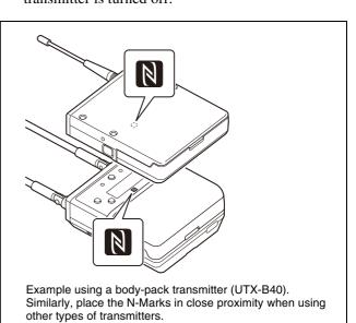
Information about the channel and compander mode set on the tuner are sent to the transmitter, and then the transmit channel is set.
