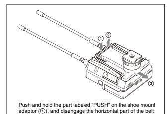
clip from the horizontal groove on the shoe mount adaptor (②). Then, push the shoe mount adaptor in the direction of
